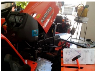
Figure 24. Measuring fuel consumption of Kubota D1703-M-DI engine.
